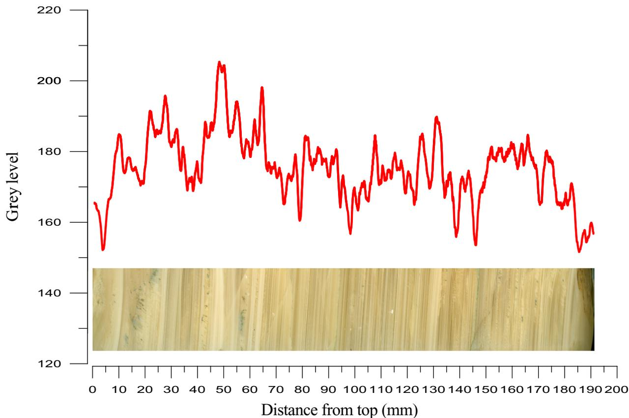
Fig. 2. Plot of grey level of stalagmite BW-1 versus distance from the top. The stalagmite section is shown at the bottom for comparison. The high grey level values match the milk-white coloured intervals, whereas the low grey level values match the transparent-brown calcite locations. At the very top and bottom of the stalagmite profile, the grey level may be lower than the true values (see main text for details). This figure is available in colour at <http://www.boreas.dk>.
